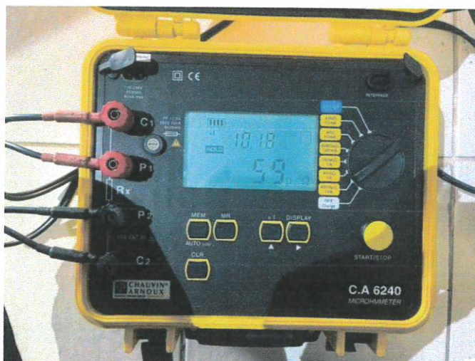
CONTACT RESISTANCE TEST
