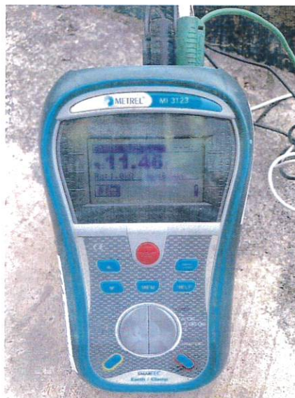
GROUNDING RESISTANCE TEST
