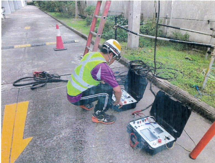
TURN RATIO AND DC WINDING RESISTANCE INSPECTION
