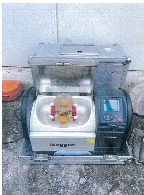
DIELECTRIC BREAKDOWN OF OIL TEST
