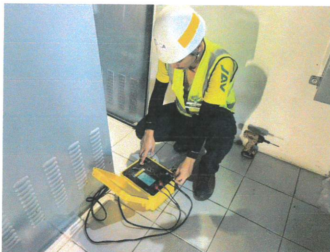
CONTACT RESISTANCE TEST
